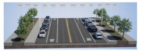
A typical cross-section for an industrial collector.
